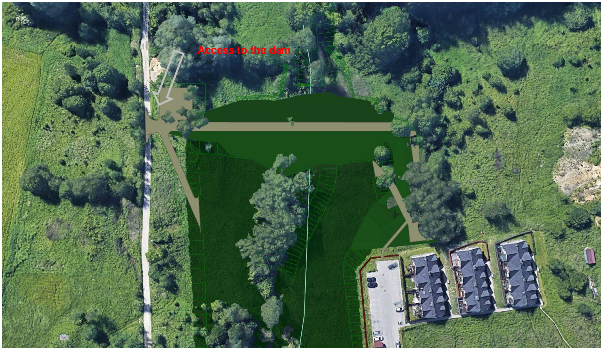
Figure 6. Planned access ways to the front dam and exits to the Malinówka 3 reservoir bowl
